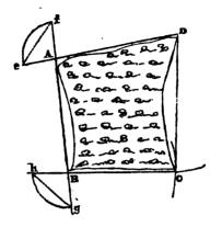
measure, on the outside of the wood, from A to B, and continue the line beyond B to g, which is 100 links: also measure out 100 links to h, in the line B C, and measure h g. Now measure B C, C D, and D A.
